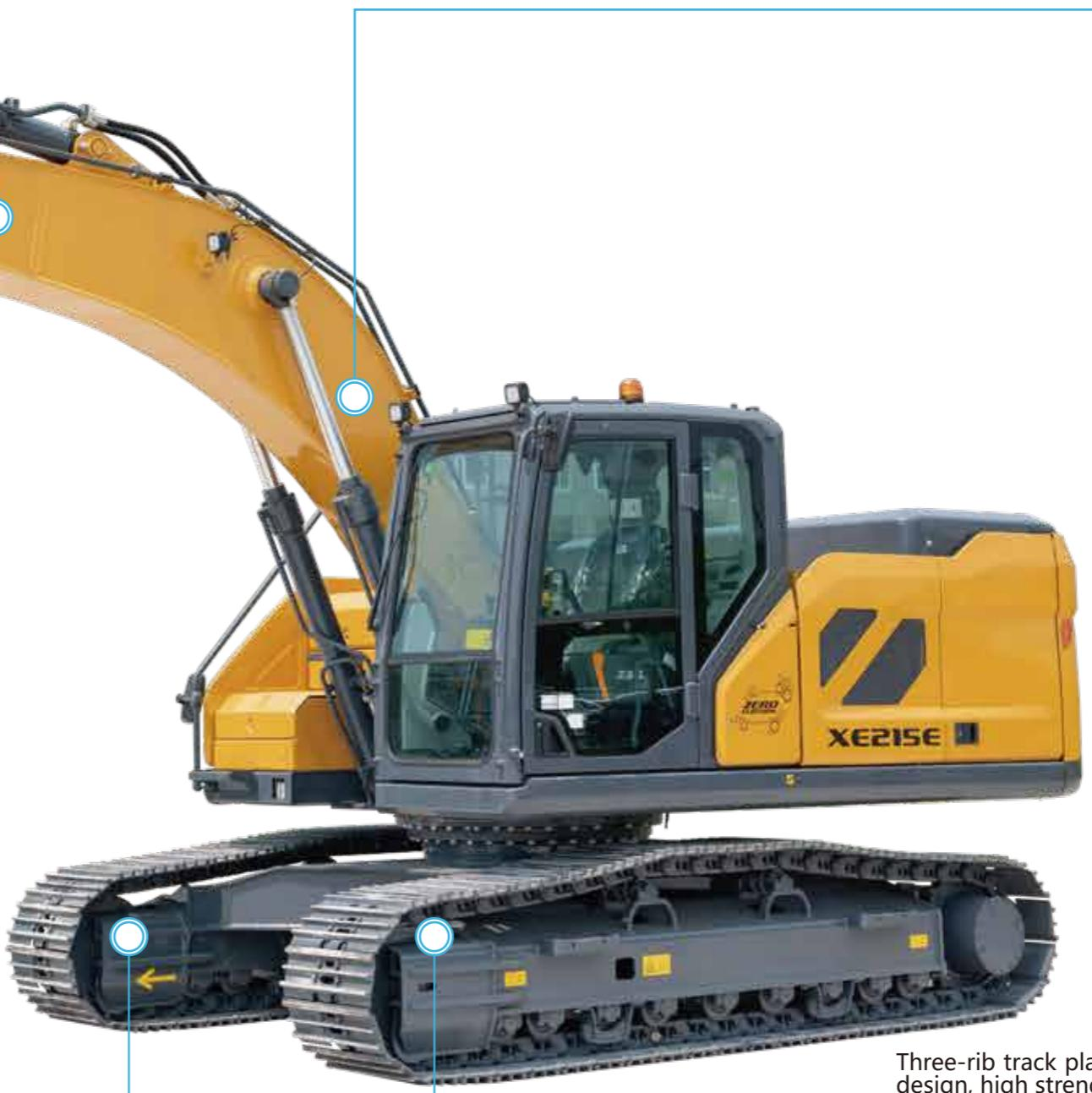
Three-rib track plate: thickened tooth root design, high strength and super grip.
