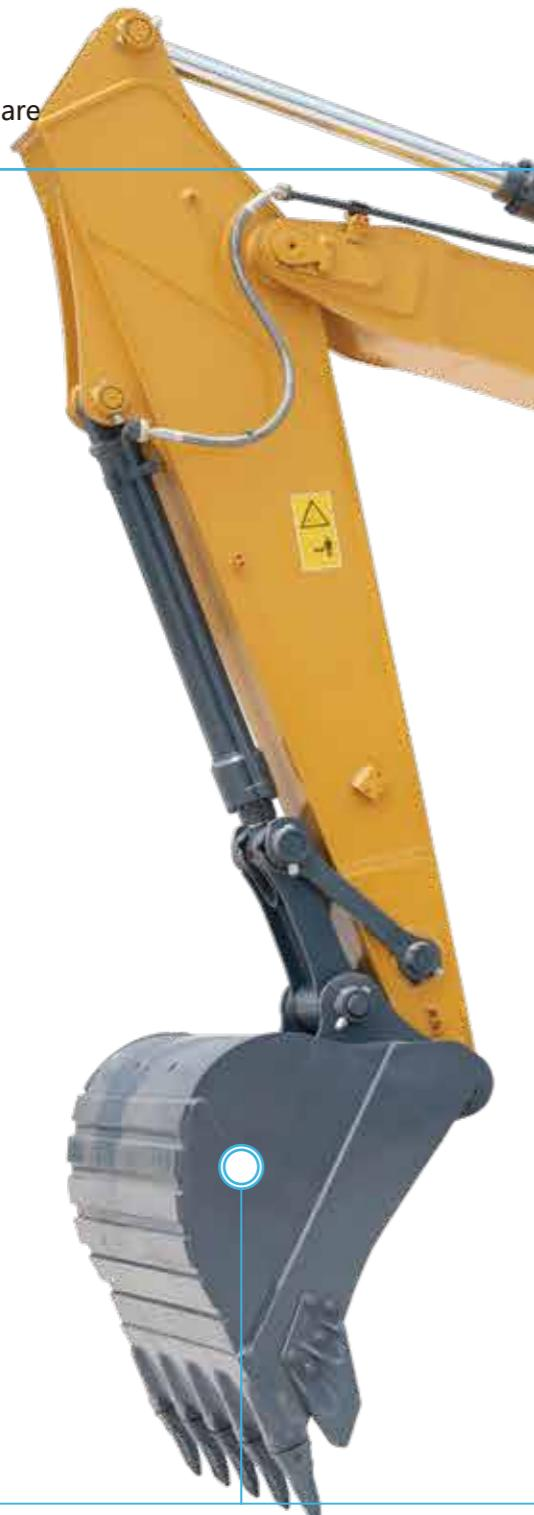
The front supports of the equipment are all made of high-strength plates welded together, and the middle and rear supports are all made of forged structure, with higher strength and longer service life.
